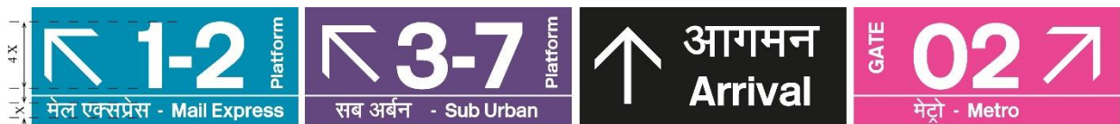
Figure 9: Colour scheme for zoning of different train type/traffic segment at complex station
